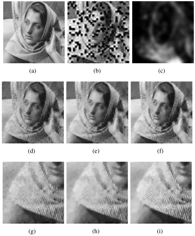
Fig. 9. Random loss of 20% of wavelet coefficients with Gaussian noise \sigma = 0.1 (a) Original image before information loss (b) Received image back-projected (c) Final values of \lambda by our adaptive parameter choice rule (d) Best PSNR-reconstruction by the primal-dual Newton algorithm ( \lambda = 20 , PSNR=22.63, MSSIM=0.676) (e) Best MSSIM-reconstruction by the primal-dual Newton algorithm ( \lambda = \frac{100}{7} , PSNR=22.58, MSSIM=0.686) (f) Reconstruction via sSA-TV method (PSNR=22.93, MSSIM=0.718). In (g) - (i) we zoomed on the scarf.
