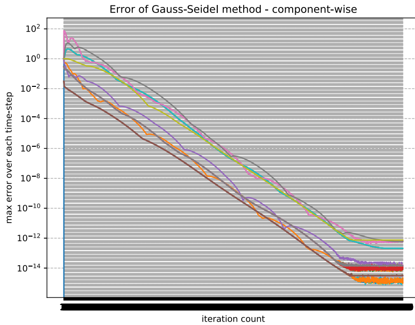
Fig. 3 Solving the bandpass filter in Fig. 3 using (58)-(60). The plot shows error for each iteration's error.
