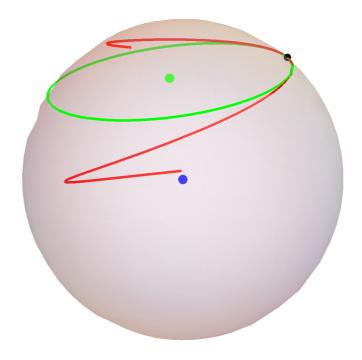
This picture shows a piece of a curve (red), one of its points (black), the osculating circle with its center (green), and the osculating sphere with its center (blue) at this point, see subsection 4.2.
