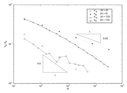
Fig. 6. Error estimator and approximated error for uniform ( $\Theta = 0$ ) and adaptive ( $\Theta = 1/2$ ) mesh-refinement in Example 5.3.
