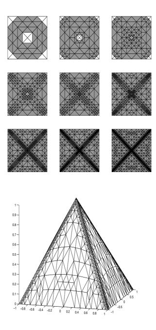
**Fig. 5.** Adaptively refined meshes  $\mathcal{T}_0$  (left upper) to  $\mathcal{T}_8$  (right lower) (top) with approximate discrete contact zone shown in white and solution  $u_h$  on  $\mathcal{T}_8$  with 1149 free nodes (bottom) in Example 5.3.
