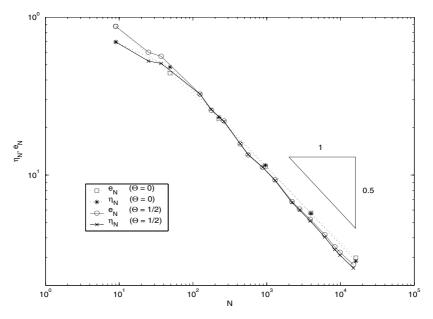
Fig. 2. Error and error estimator for uniform ( $\Theta = 0$ ) and adaptive ( $\Theta = 1/2$ ) mesh-refinement in Example 5.1.
