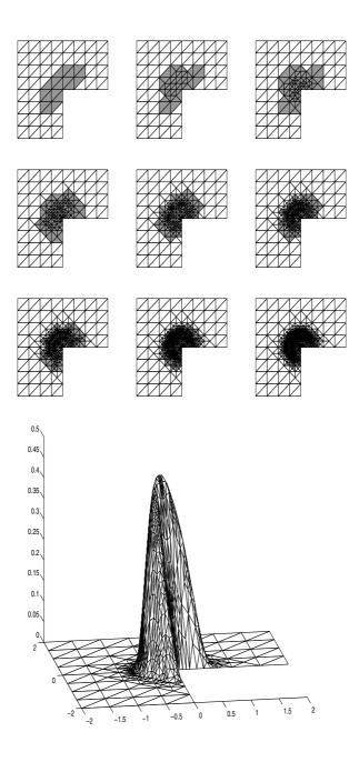
**Fig. 3.** Adaptively refined meshes  $\mathcal{T}_0$  (left upper) to  $\mathcal{T}_8$  (right lower) (top) with approximate discrete contact zone shown in white and solution  $u_h$  on  $\mathcal{T}_8$  with 572 free nodes (bottom) in Example 5.2.
