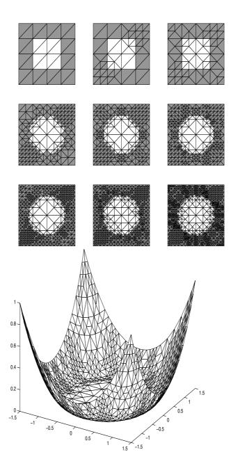
**Fig. 1.** Adaptively refined meshes  $\mathcal{T}_0$  (left upper) to  $\mathcal{T}_8$  (right lower) (top) with approximate discrete contact zone shown in white and solution  $u_h$  on  $\mathcal{T}_8$  with 881 free nodes (bottom) in Example 5.1.
