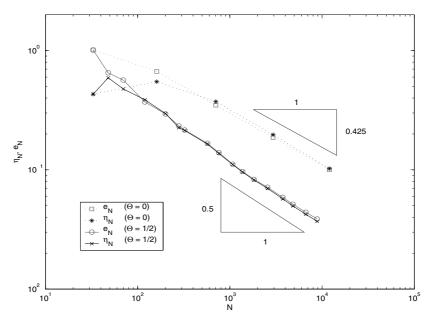
Fig. 4. Error and error estimator for uniform ( $\Theta = 0$ ) and adaptive ( $\Theta = 1/2$ ) mesh-refinement in Example 5.2.
