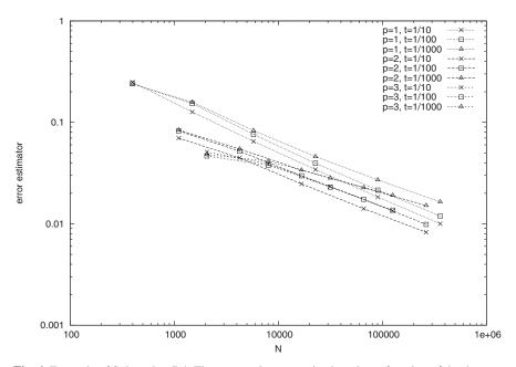
**Fig. 4** Example of Subsection 7.4: The error estimator  $\eta_R$  is plotted as a function of the degrees of freedom *N* for polynomial degrees p = 1, 2, 3, thickness'  $t = 10^{-k}$  for k = 1, 2, 3, and for uniform mesh refinement
