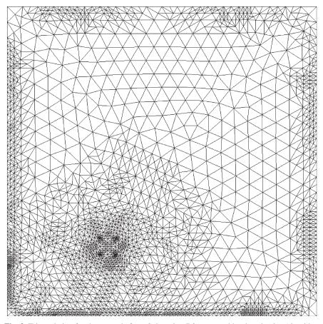
**Fig. 3** Triangulation for the example from Subsection 7.3 generated by the adaptive Algorithm (A) with 5267 element domains with p = 3, N = 206961 degrees of freedom, and thickness t = .01. One observes some balance of local mesh-refining towards the outer boundaries (for boundary layer resolution) and towards the vertices of the stamp with discontinuities of the applied load
