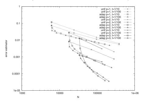
**Fig. 2** Example of Subsection 7.3: The error estimator  $\eta_R$  is plotted as a function of the degrees of freedom N for polynomial degrees p = 1, 2, 3, thickness'  $t = 10^{-k}$  for k = 1, 2, and for uniform and adaptive mesh refinements
