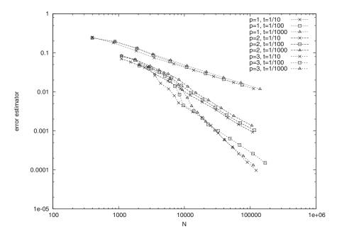
**Fig. 5** Convergence history for the example of Subsection 7.4 with the adaptive Algorithm (A), where the error estimator  $\eta_R$  is plotted as a function of the degrees of freedom *N* for polynomial degrees p = 1, 2, 3 and thickness'  $t = 10^{-k}$  for k = 1, 2, 3 and for adaptive mesh refinement
