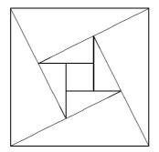
Fig. 1.1. Mesh excluded from this paper as it is not partly red-refined from some regular mesh  $\mathcal{T}_0$ . The degree of hanging nodes in the displayed mesh is hard to specify and patches of free nodes can contain an unbounded number of elements (since the figure can be extended in a self-similar sense).
