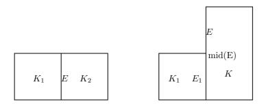
No hanging node on E Hanging node mid(E). Fig. 2.2. Edges without (left) resp. with (right) hanging node.
