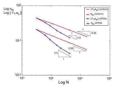
Fig. 5.3. Experimental convergence rate of  $\eta_N$  and the exact error  $\|\nabla_h e_N\|$  with respect to the number N of degrees of freedom for the adaptive and uniform refinement based on  $\eta_N$  and with the  $N\!R$  finite element.
