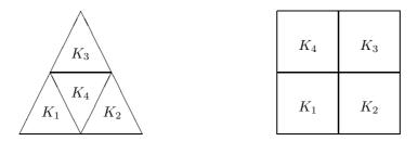
Fig. 2.1. Red-refinement of element domain  $K = K_1 \cup K_2 \cup K_3 \cup K_4$  into 4 congruent subdomains  $K_1, \ldots, K_4$  in case of a triangle (left) and a parallelogram (right): red $(K) = \{K_1, \ldots, K_4\}$ .
