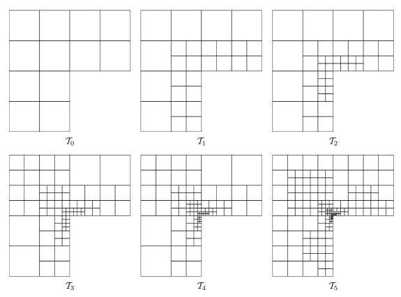
Fig. 5.2. Adapted triangulations  $\mathcal{T}_0, \ldots, \mathcal{T}_5$  generated with the Algorithm 5.1 with  $\theta = 1/2$ .
