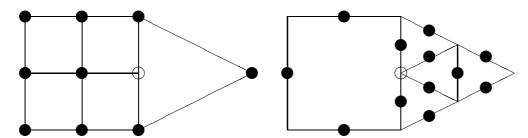
Fig. 5.1. Triangulation with conforming (left) and nonconforming (right)  $P_1$  and  $Q_1$  elements and one hanging edge  $E_H = E_{H,1} \cup E_{H,2}$ .
