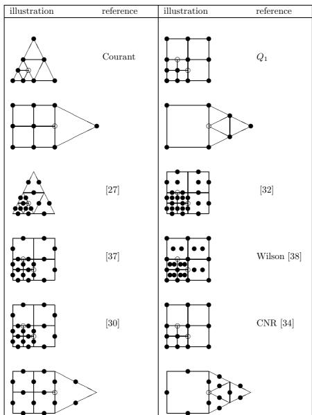
Table 1.1: FEMs with hanging nodes: bullets mark the degrees of freedom and circles mark hanging nodes subsect to internal restrictions.
