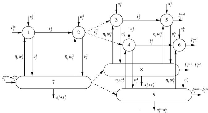
Fig. 9. Example network for hydro-storage plant  $j$
